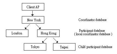
Figure 15-3 DBMaker distribution structure
