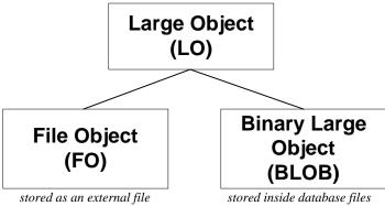
Figure 7-1: Large Objects supported by DBMaker
