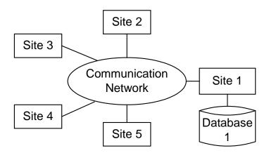
Figure 15-1 Traditional client/server database management system
