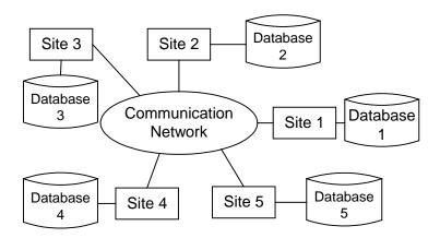
Figure 15-2 Distributed database in client-server
