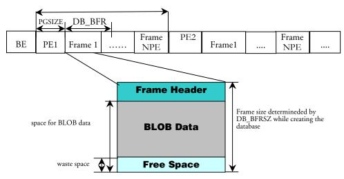
Figure 7-3: the structure of a BLOB file
