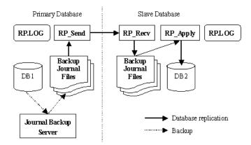
Figure 16-11: Flow of database replication
