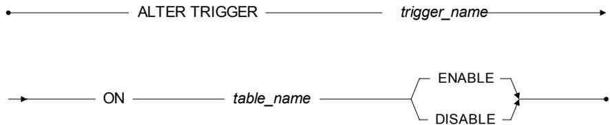
Figure 3-24 ALTER TRIGGER ENABLE syntax
