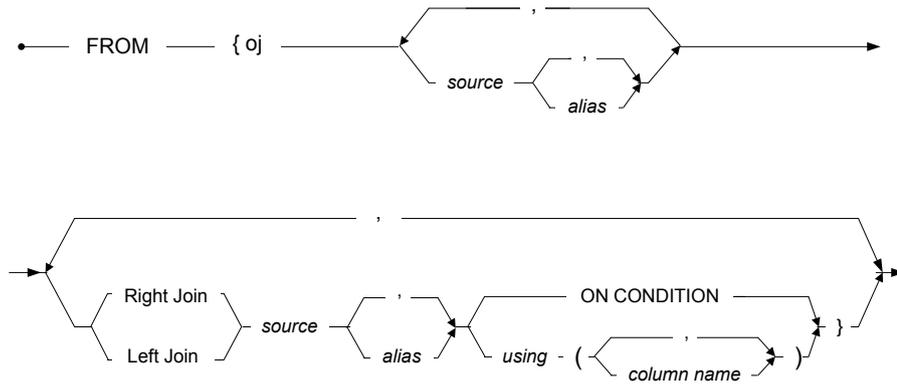
Figure 3-116 ODBC Outer-Join Syntax
