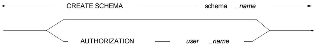
*Figure 3-46 CREATE SCHEMA syntax*
