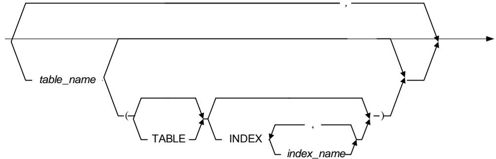
Figure 3-141 UNLOAD STATISTICS Object List syntax
