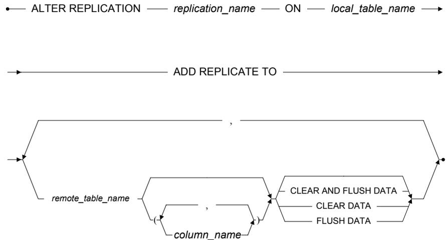
Figure 3-7 ALTER REPLICATION ADD REPLICATE syntax
