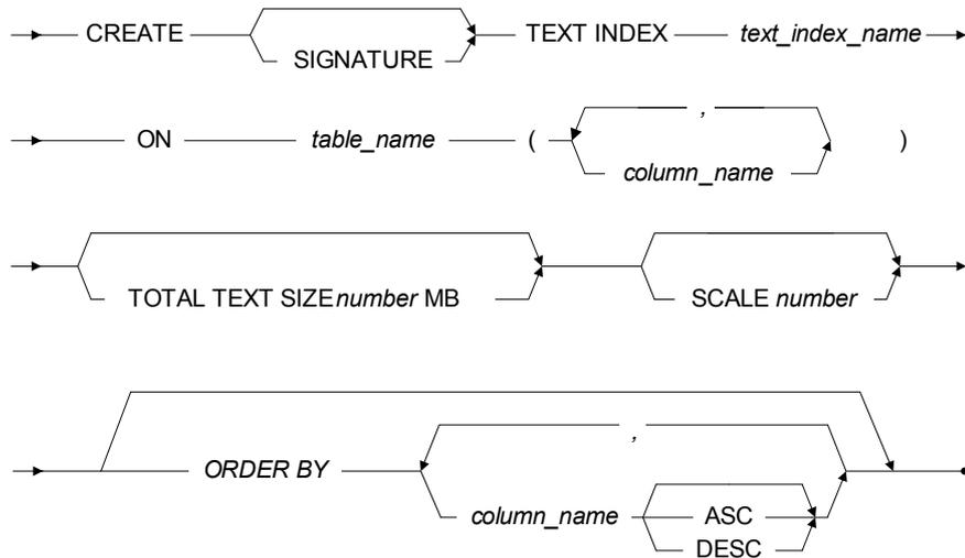
Figure 3-55 CREATE SIGNATURE TEXT INDEX syntax
