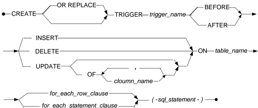
Figure 3-57 CREATE TRIGGER syntax
