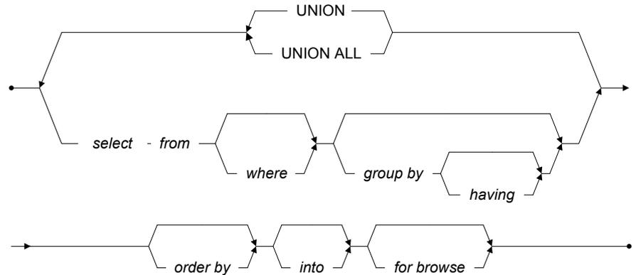
*Figure 3-98 SELECT (using FROM) syntax*
