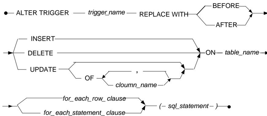
Figure 3-25 ALTER TRIGGER REPLACE syntax
