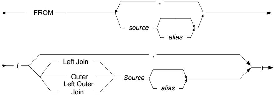
*Figure 3-115 DBMaker Outer-Join Syntax*
