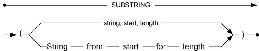
Figure 4-112 SUBSTRING syntax
